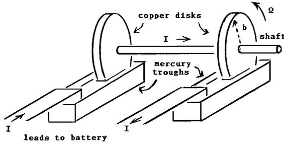
Fig. 3 – Proposed motor with copper disks and shaft, that replace the wire bridge of Ampère’s original experiment, connected electrically in two mercury troughs.
