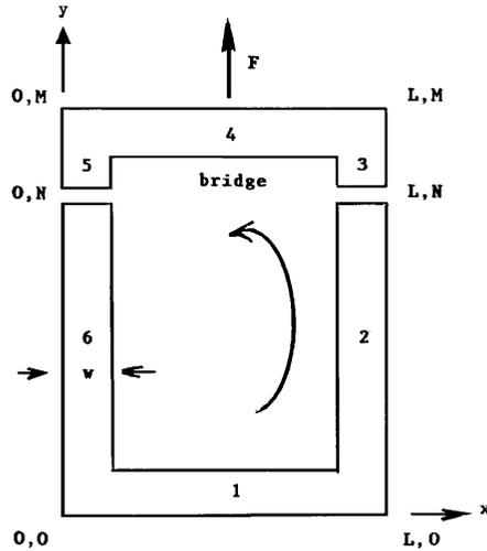
Fig. 1 – Diagram for the Ampère bridge experiment indicating the geometry and choice of coordinates for rectangular leads of width  $w$  and thickness  $t$ .
