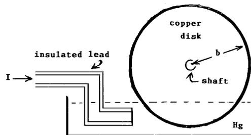
Fig. 4 – Diagram of one of the mercury troughs indicating how the current lead can delivery current tangentially to the under rim of the disk.
