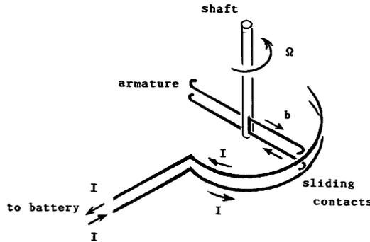
Fig. 2 – Diagram of the proposed motor driven by the Ampère repulsion between colinear current elements to illustrate the electrical principle. Insulated leads are matched by immediately adjacent leads carrying current in the opposite direction.
